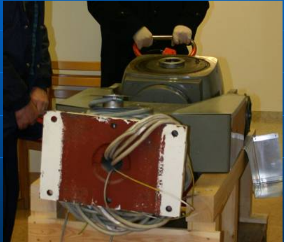
A dismantled Co treatment head
